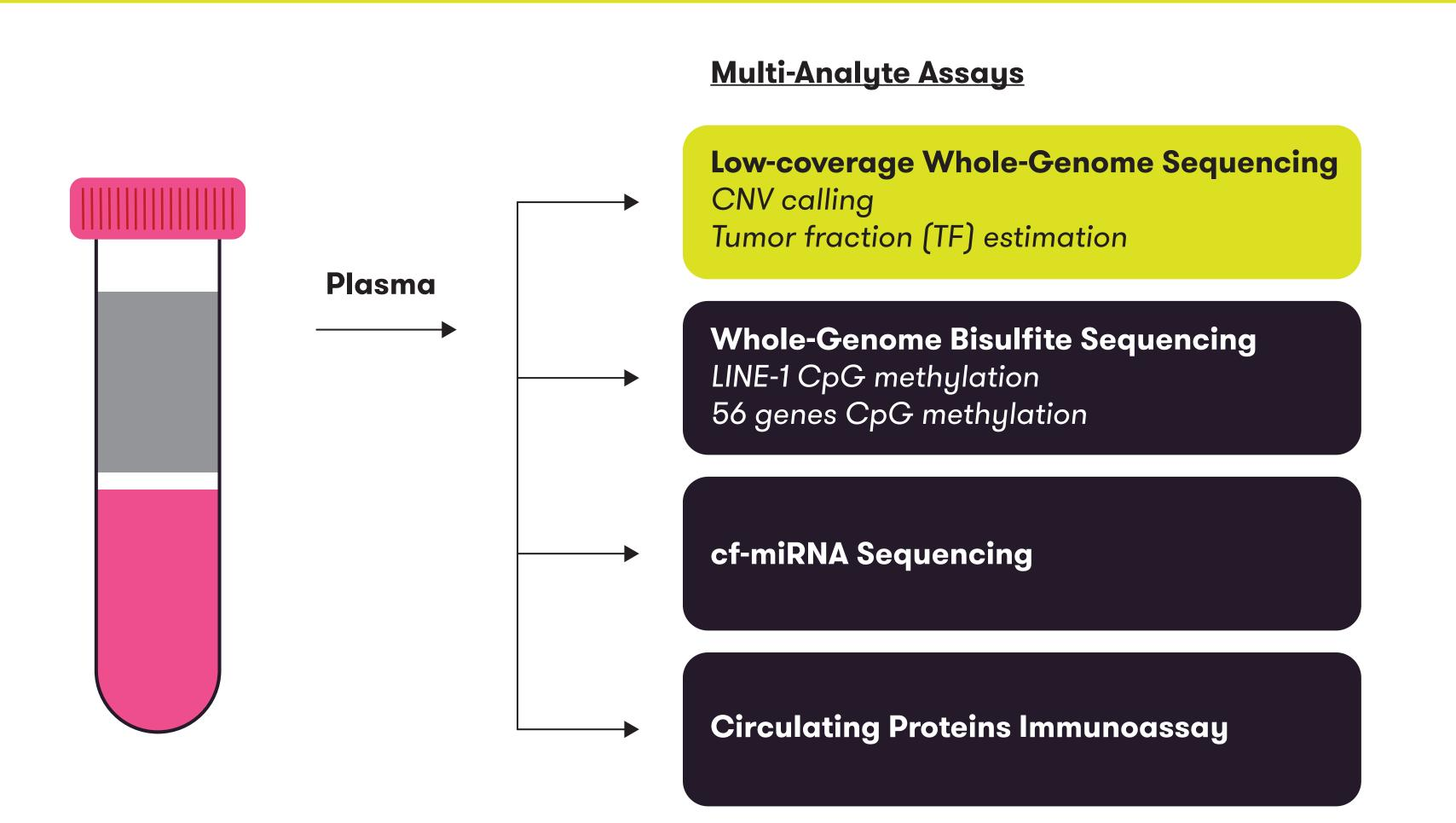
ollected in K3-EDTA tubes, and double-spun to isolate plasma. Plasma was split into aliquots for cfDNA lcWGS, WGBS, cf-miRNA sequencing, and quantitative immunoassays. CNV, copy number variation; LINE-1, long interspersed nuclear element 1.
